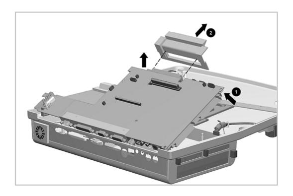
Figure 7-20. Removing the Main Board Assembly
